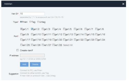
2.Permitted VLAN pass through Trunk port. Click the navigation tree "Business Management > VLAN > Port-vlan" menu, input VLAN ID of VLAN which is allowed pass through Trunk port, select the appropriate interface among Tag port list, click "add" to complete the configuration
