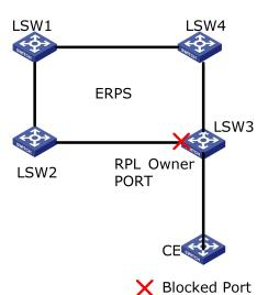
ERPS ring, that is, by a group configured with the same control VLAN Layer 2 switching equipment constituted, is the basic unit ERPS agreement to join the second floor ERPS ring switching device called a node. Each node can not join more than two ports with a ERPS ring, join node needs to be configured to add.
