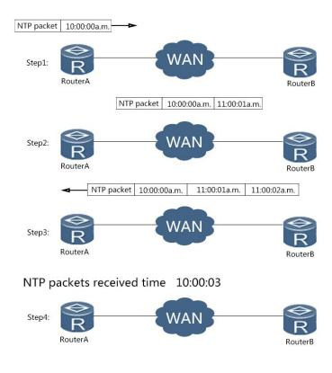
System clock synchronization process is as follows:
